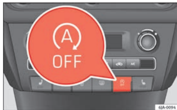
Abb. 111 Kombi-Instrument: Taster START-STOPP-System .
